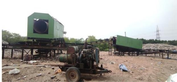
**FIGURE 3.2:** Waste segregation or sorting machine
